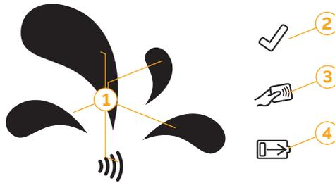
The LED information panel indicates the device's operating status. Standby, charging, waiting, and fault condition is indicated by the corresponding four symbols lighting up in the display.
